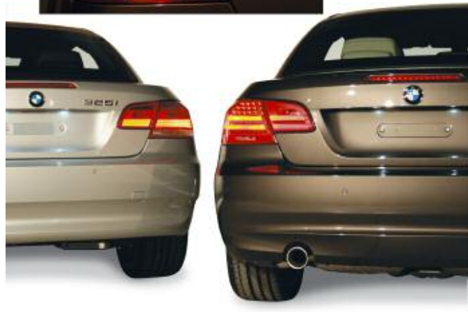
92/E93 comparison: Predecessor at left, LCI rear lights in LED technology at right and top
